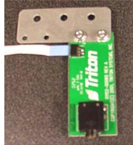
6. Insert audio board assembly to the control panel and start the right side screw using the K40x12 screws included. Connect/secure the cable routing clip shown on the left side screw hole. Tighten both screws.
