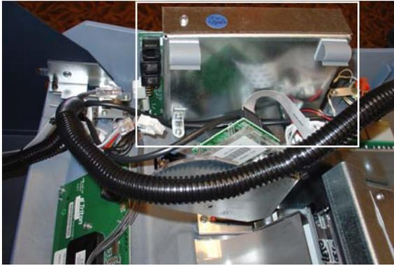
2. Remove the phillip-head screws that secure the Main board assembly to the control panel (Figures below). Set screws aside. *Note: There may be a ground wire attached under the screw for the L-bracket.*
