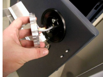
Figure 3. Insert keypad cable through hole in mounting plate. Align large holes in keypad mounting slots with shoulder screws on mounting plate.
