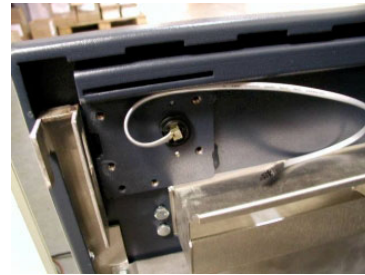
Figure 7. Cable curves over top of bushing and exits to the right, as shown.
