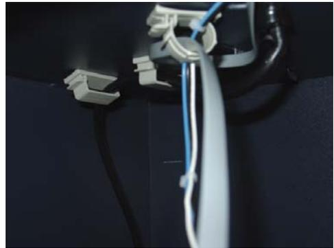
Figure 27. Route cables through clip.
