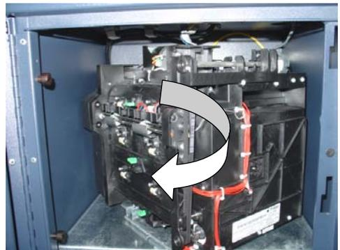
Figure 2. Rotate dispenser clockwise.
