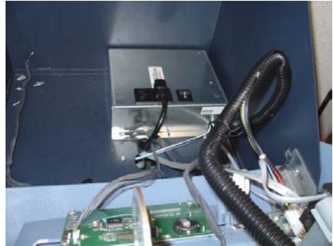
Figure 26. Cables connected w/tubing.
