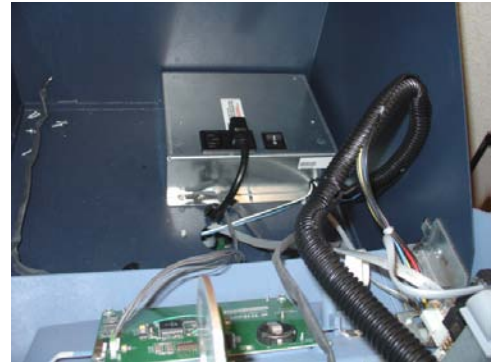
Figure 26. Cables connected w/tubing.
