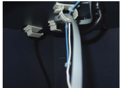
Figure 27. Route cables through clip.
