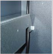
2. This step involves assembling the slide rails to the tray mounting brackets. There are 2 different slide rails: **locking** (mounted on right side) and **non-locking** (mounted on left side). Figure 2 shows the locking slide rail. To assemble, slide the rail out fully as shown in Figure 2. Align the mounting bracket with the three (3) holes pictured (Figure 3) and secure them together using three (3) truss head phillip screws (P/N 02054-00048). Repeat for the other slide rail/bracket.
