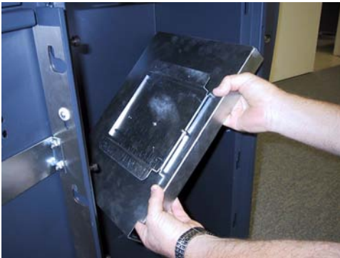
Figure 8. Turn tray to clear door edges.
