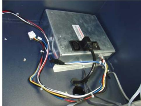
*Figure 1. DC power cables disconnected..*
