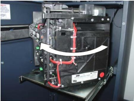
*Figure 3. Rotate mechanism to service position (clockwise).*
