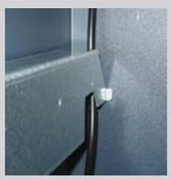
2. This step involves assembling the slide rails to the tray mounting brackets. There are 2 different slide rails: **locking** (mounted on right side) and **non-locking** (mounted on left side). Figure 2 shows the **locking** slide rail. To assemble, slide the rail out fully as shown in Figure 2. Align the mounting bracket with the three (3) holes pictured (Figure 3) and secure them together using three (3) truss head phillip screws (P/N 02054-00048). Repeat for the other slide rail/bracket.
