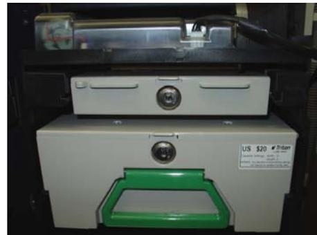
*Figure 3. Mechanism in service position.*
