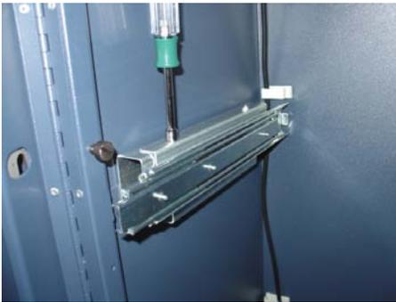
Figure 7. Remove nuts from mounting bracket.
