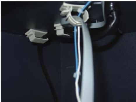
Figure 6. Route cables through clip.
