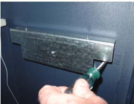
Figure 9. Remove nuts from mounting bracket.
