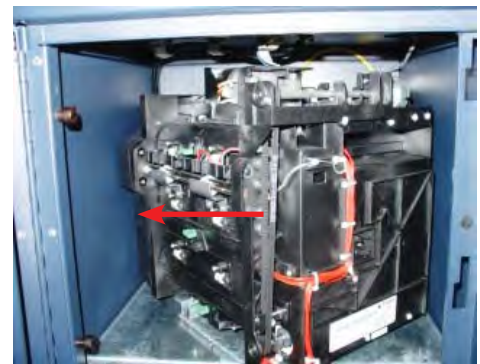
Figure 2. Rotate dispenser clockwise.
