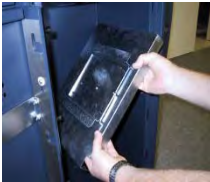
Figure 8. Turn tray to clear door edges.
