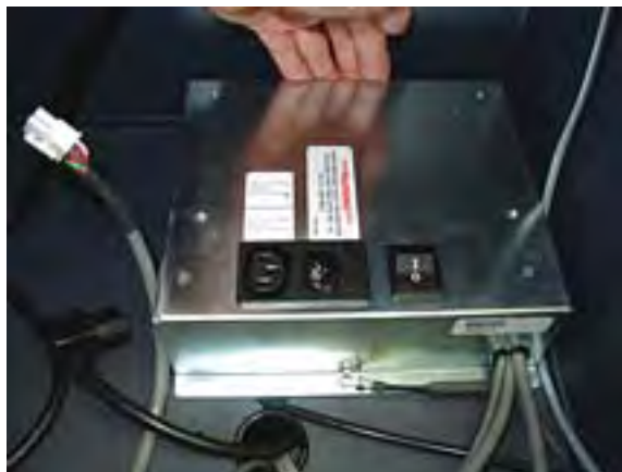
Slide the single power supply forward and lift it from the cabinet top enclosure
