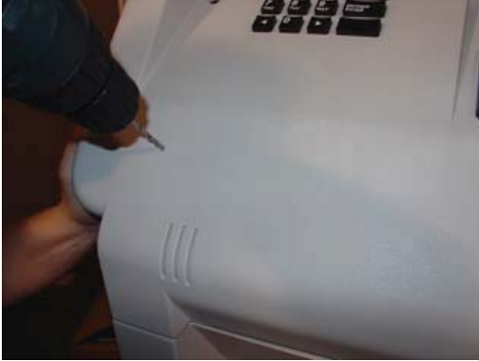
Figure 4. Drill pilot hole.
