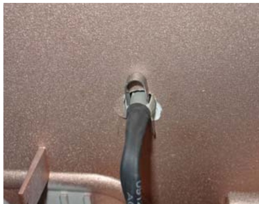
Figure 8. Insert retainer clip to secure.
