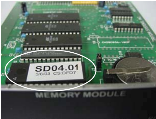
Figure 14. Memory module EPROM location.
