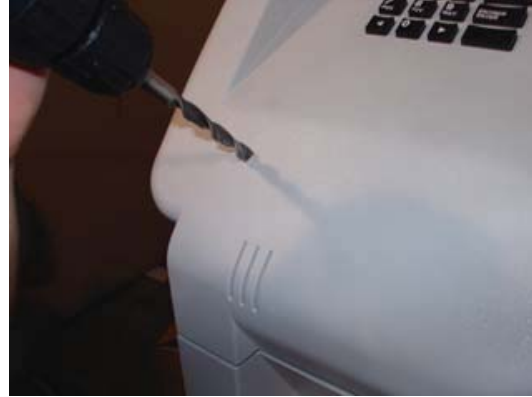
Figure 5. Finish with 7/16" bit.
