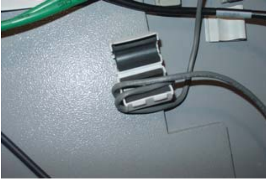
Figure 17. Install cable in ferrite.
