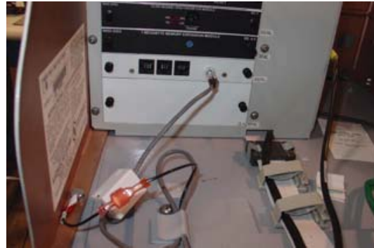
Figure 18. Connect cable to Multi function board.
