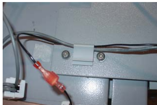
Figure 12. Install flat clip and secure cable.
