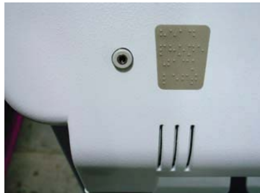
Figure 7. Headphone plug flush.
