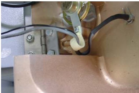
Figure 11. Install clip and route cable.
