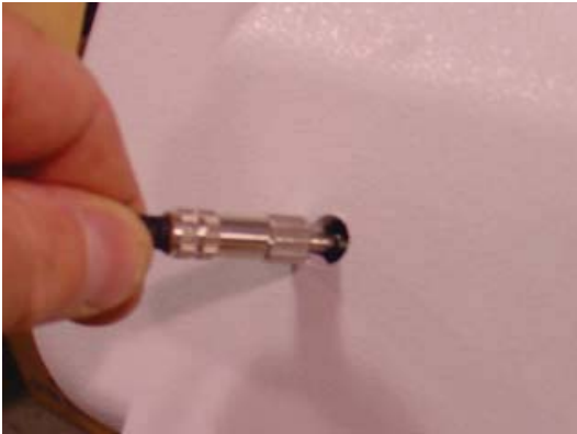
Figure 6. Feed cable in hole.
