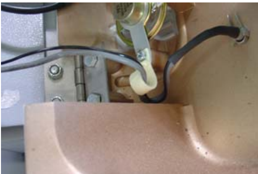
Figure 11. Install clip and route cable.
