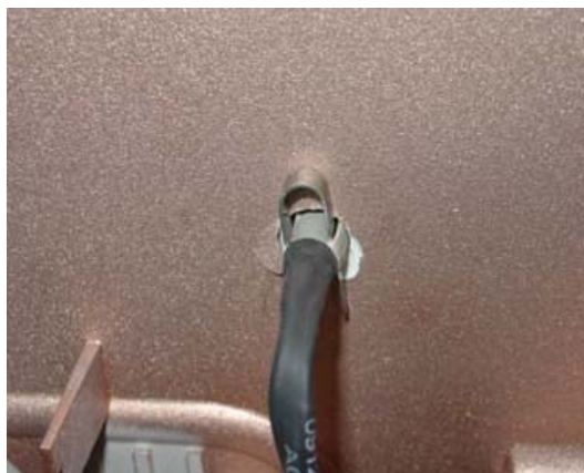
Figure 8. Insert retainer clip to secure.
