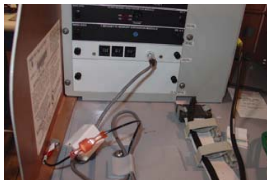
Figure 18. Connect cable to Multi-function module.
