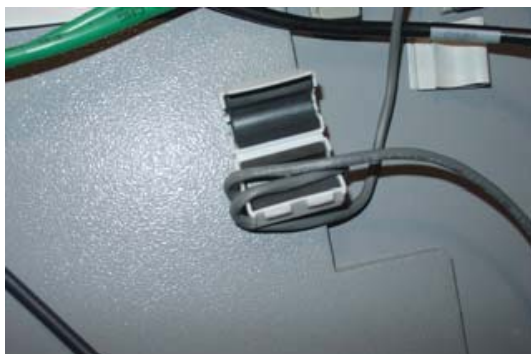
Figure 17. Install cable in ferrite.
