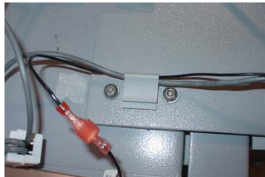
Figure 12. Install flat clip and secure cable.
