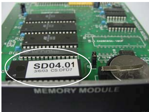
Figure 14. Memory module EPROM location.
