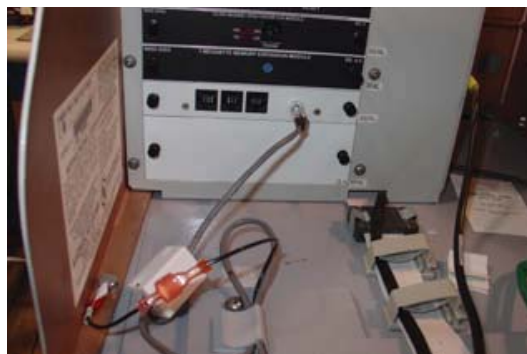
Figure 18. Connect cable to Multi-function module.
