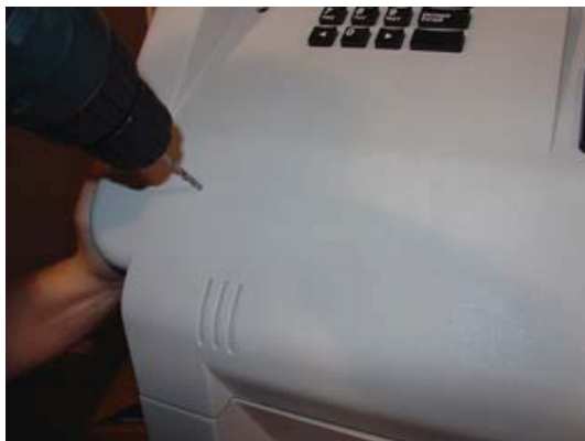
Figure 4. Drill pilot hole.
