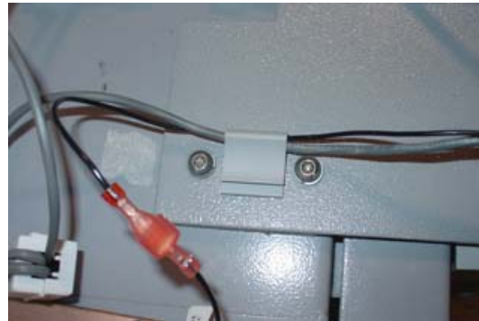
Figure 12. Install flat clip and secure cable.
