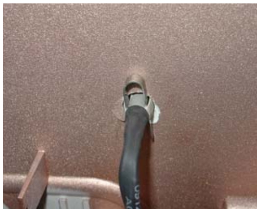
Figure 8. Insert retainer clip to secure.
