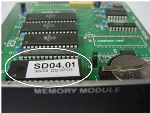
Figure 14. Memory module EPROM location.
