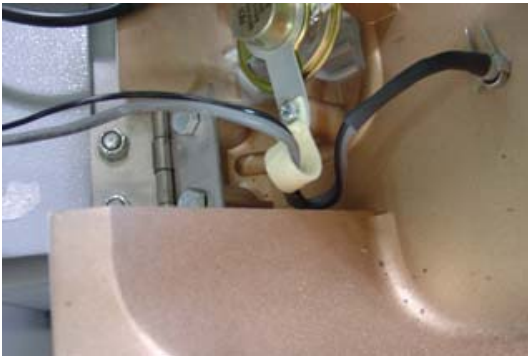
Figure 11. Install clip and route cable.
