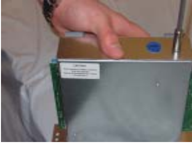
Figure 2-22a. Top screw location.
