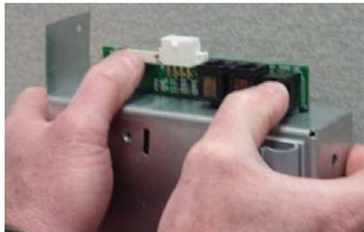
Figure 2-23b. Housing separation.
