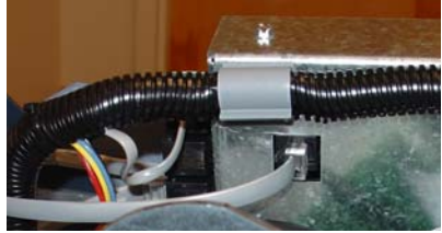
Figure 2-36. (RS-232) RJ-45 connection.
