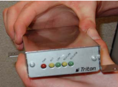
Figure 2-31. Mount external Ethernet bracket.
