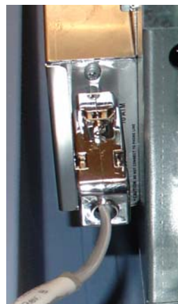
Figure 2-35. (RS-232) 9-pin connection.
