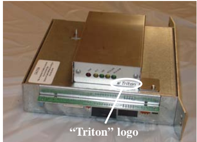
Figure 2-32. Install Ethernet assembly and bracket to mounting screws.
