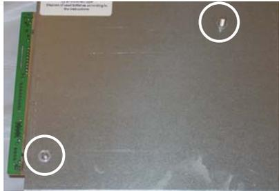
Figure 2-27. Protruding screws.
