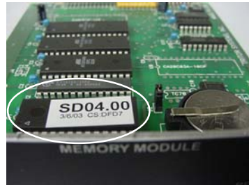
Figure 2-13. Memory module EPROM location.
