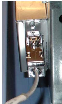
Figure 2-35. (RS-232) 9-pin connection.
