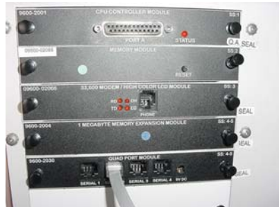
Figure 2-18. RJ-45 connected to Serial 2 of Quad Port module.
