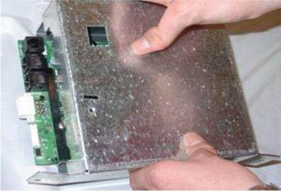
Figure 2-29. Install Main board housing w/Ethernet adapter cutout.
