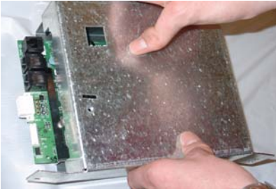
Figure 2-29. Install Main board housing w/Ethernet adapter cutout.
