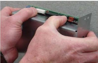
Figure 2-23a. Housing separation.
