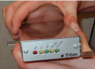
Figure 2-31. Mount external Ethernet bracket.
