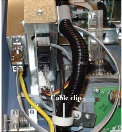
*Figure 2-37. External Ethernet cables routed and connected.*
