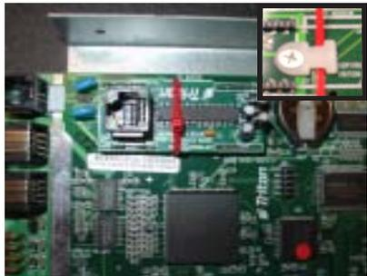
Figure 2-28. Install Ethernet adapter.
