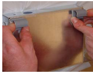
Figure 2-34. Affix cable clips.
