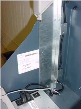
Figure 6. Route power cable behind bracket.
