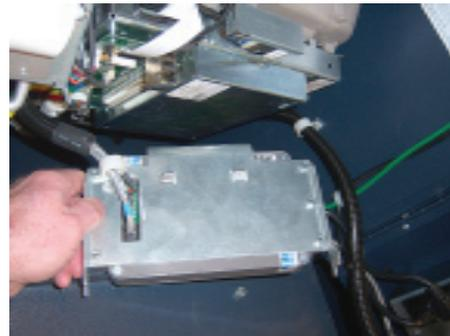
➤ Place the EPP assembly on a flat surface. Remove the six (6) screws/nuts that secure the EPP to the mounting bracket. Retain the screws and cable guide. Both the T7 (PCI-EPP) and the T5 (PCI-EPP) require this new bracket (included in kit) when installed in the RT2000.
