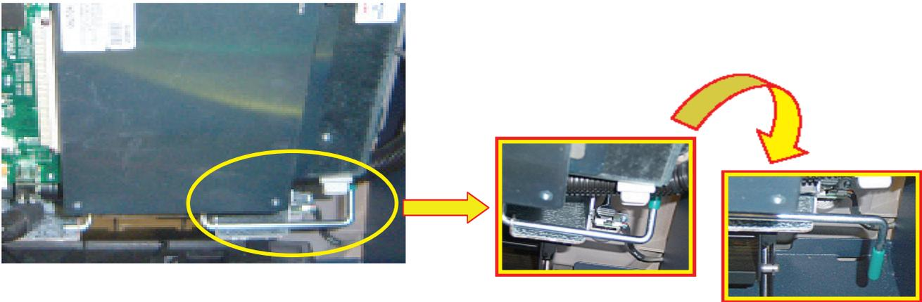
➤ Carefully remove the EPP and its mounting bracket. When the assembly is clear of the Control panel, turn it over and disconnect the Function key cable(s) and RJ45 data cable. Remove the EPP module and mounting bracket from the ATM.
