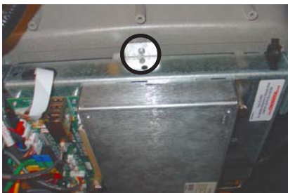
Figure 2. Secure bracket to screw shown.
