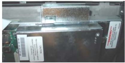
Figure 3. Modem bracket mounted.
