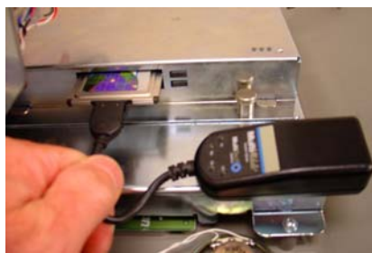
Figure 2. Remove PCMCIA modem card and adapter.
