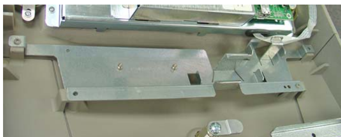
Figure 3. Install modem mounting bracket.
