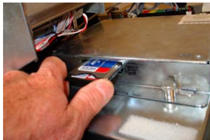
Figure 2. Insert into PCMCIA slot.
