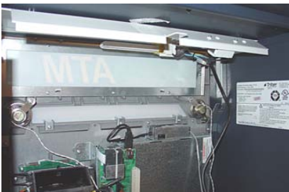
BALLAST/BULB LIGHT PANEL
