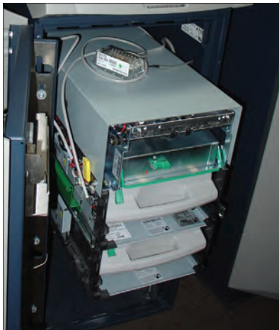
At left: The NMD 50 with dual cassettes. At right: RL unit converted to incorporate the SDD dispenser. Some SDDs attach to fixed-base units, while others are mounted on sliding decks. Below: Metal SDD cash cassette fits all SDD units.
