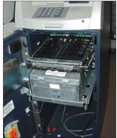
At left: The NMD 50 with dual cassettes. At right: RL unit converted to incorporate the SDD dispenser. Some SDDs attach to fixed-base units, while others are mounted on sliding decks. Below: Metal SDD cash cassette fits all SDD units.
