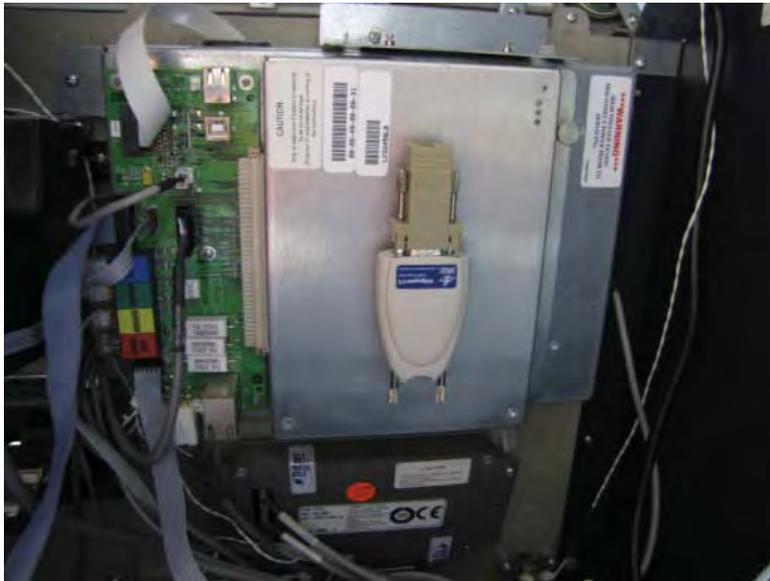
9. Obtain the Serial Modem. Notice the two slots in the back of the modem.
