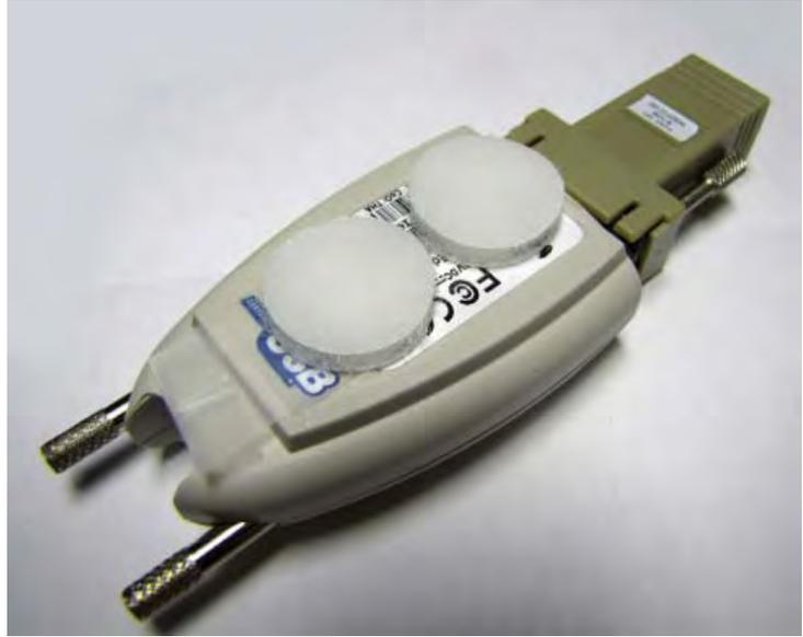
8. Adhere the Modem Assembly to the main board cover with the USB port facing down as shown.
