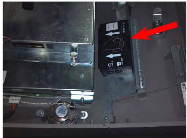
6. Plug the phone cable into the modem oLine Inö port.
