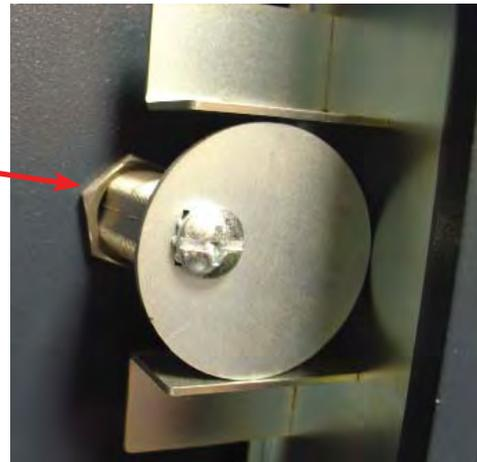
4. Position the new lock as shown (locked) and insert into the door. Hold the lock assembly as shown to ensure the tumbler mechanism does not come out throughout the rest of the installation. Secure the lock with the nut provided.
