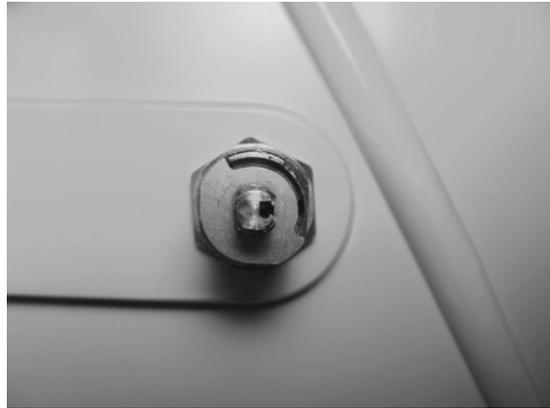
3. Maintain the hold on the key, carefully remove the stop washer, flip it over, and reinstall. It should appear as the picture at the right.
