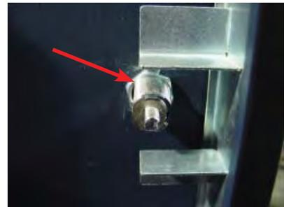
5. Remove the nut from the end of the lock. Ensure the lock stop plate stays correctly positioned, and the tumbler mechanism does not come out the front.
