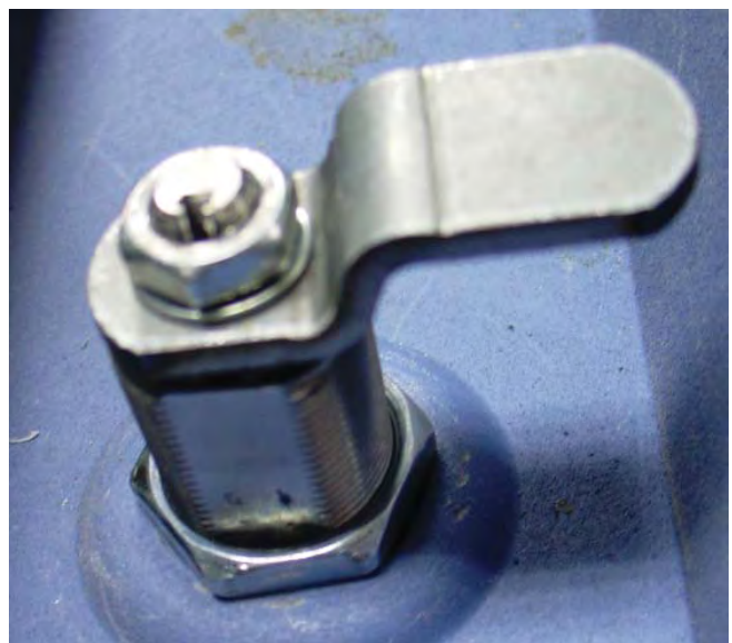
Representative lock/hasp installation, 9100 shown in the locked position.
