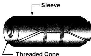
2. See **Figure 8**. The top of the expansion anchor sleeve must be flush with the mounting surface. The top cone-wedge will project slightly above the mounting surface, as shown.
