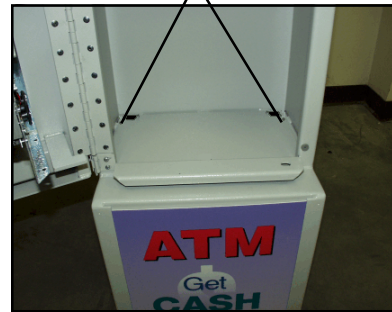
Fig. 1. Floor-Plate In Place.
