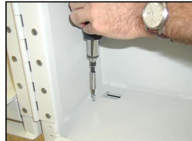
Fig. 2. Unscrewing Retaining Screws.
