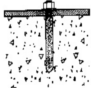
Allow seated anchor to cure.
