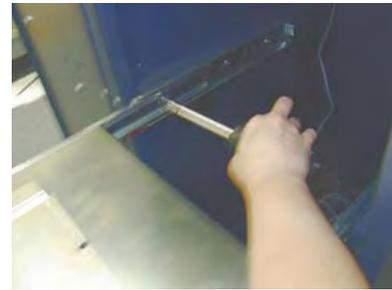
Figure 11. Remove slide rails w/tray.
