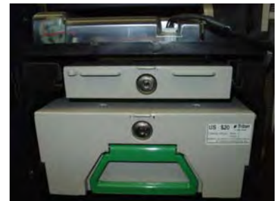
Figure 8. Mech in "Service" position.
