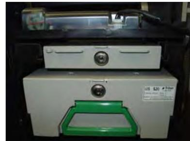
Figure 8. Mech in "Service" position.
