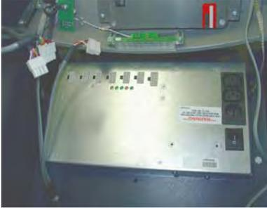
Figure 1. Disconnect all cables from power supply.
