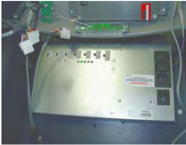
Figure 1. Disconnect all cables from power supply.
