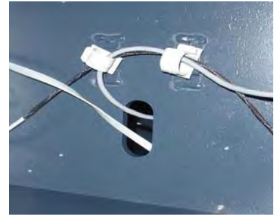
Figure 13. Route power/data cables.
