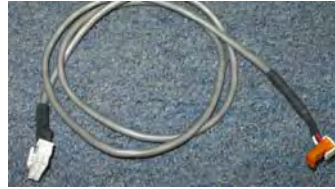
Dispenser power cable
