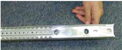
Figure 1. Slide rail extended.
