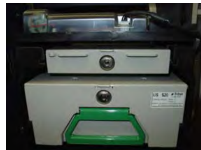
Figure 8. Mech in "Service" position.
