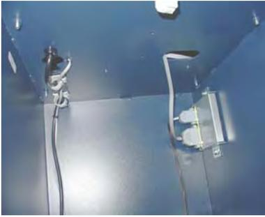
Figure 12. EJ to Docking board cable.
