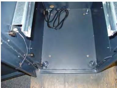
Figures 7 and 8. Slide rails flush w/bracket front.
