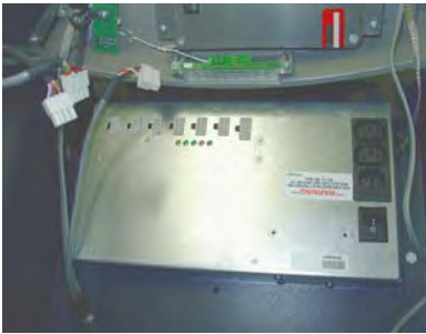
Figure 1. Disconnect all cables from power supply.
