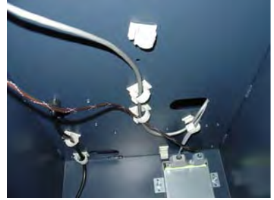
Figure 11. Route power/data cables.
