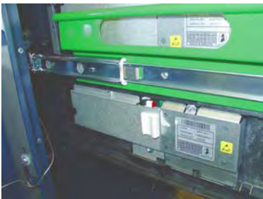
Figure 12. Insert mechanism to rail stop.
