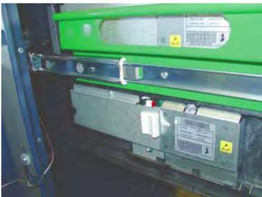
Figure 12. Insert mechanism to rail stop.
