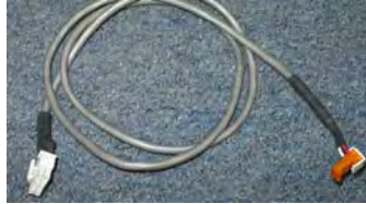
Dispenser power cable
