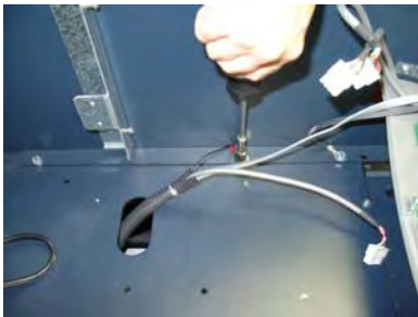
Figure 3. Disconnect ground wire.
