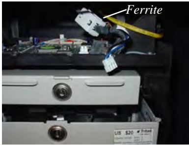
Figure 9. Power and Comm cable disconnected.
