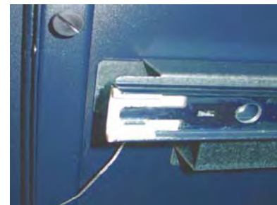
Figures 7 and 8. Slide rails flush w/bracket front.
