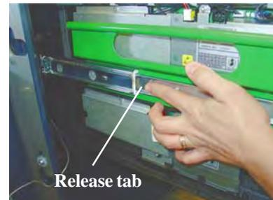
Figure 13. Push release tab.
