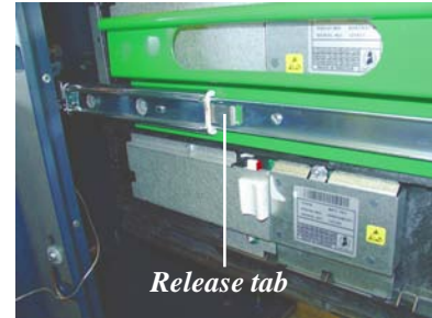
Figure 15. Push release tabs "in".
