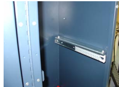
Figure 4. Assembly mounted to cabinet.
