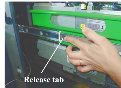
Figure 13. Push release tab.
