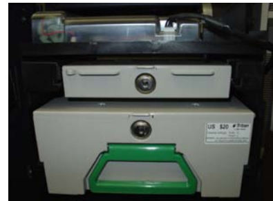
Figure 8. Mech in "Service" position.
