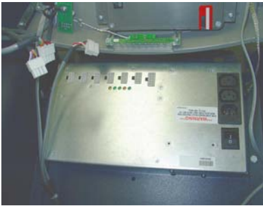
Figure 1. Disconnect all cables from power supply.
