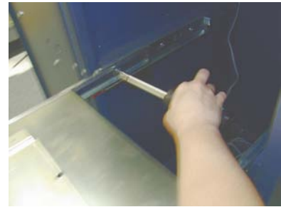
Figure 11. Remove slide rails w/tray.
