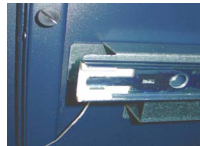
Figures 7 and 8. Slide rails flush w/bracket front.
