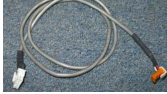
Dispenser power cable
