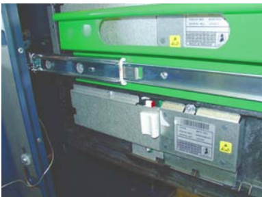
Figure 12. Insert mechanism to rail stop.
