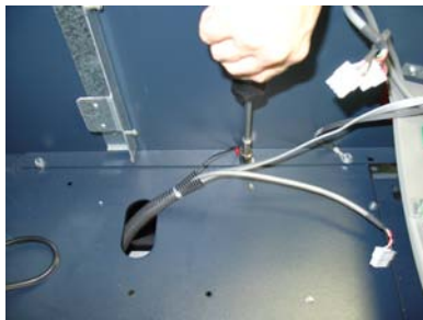
Figure 3. Disconnect ground wire.
