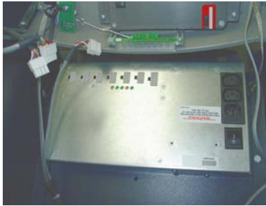
Figure 1. Disconnect all cables from power supply.
