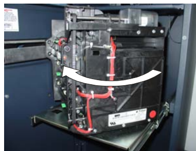
Figure 7. Rotate mechanism "clockwise".
