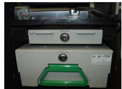
Figure 8. Mech in "Service" position.
