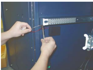
Figure 10. Remove door ground bolt.
