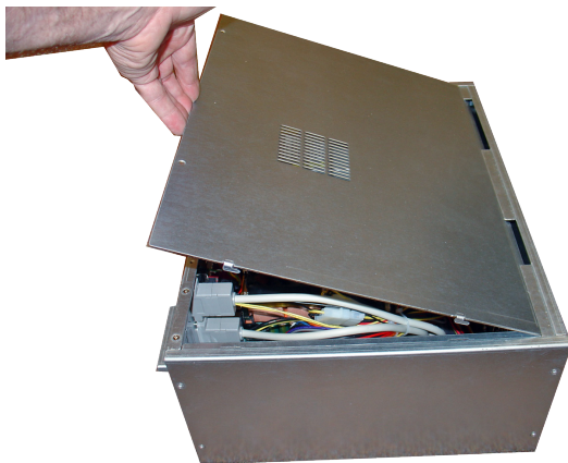
Figure 6. Removing the cover from the Controller PC assembly.
