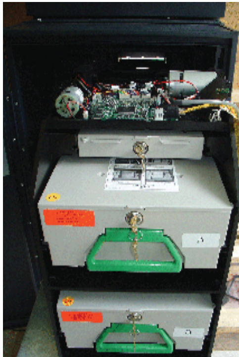
TDM-250 w/reject and note cassettes installed.
