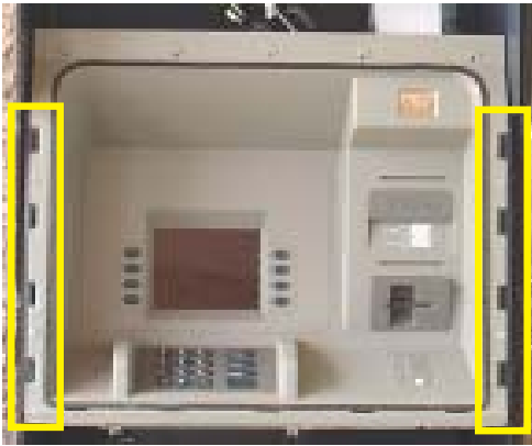
Control panel slots.
