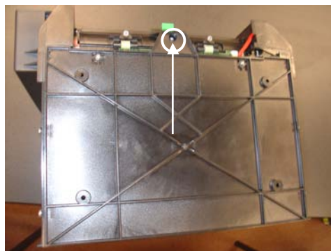
Figure 3. Bottom Torx screw location.
