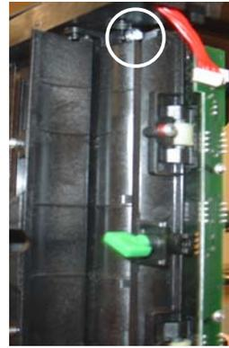
Figure 4. Open access door to locate screw.
