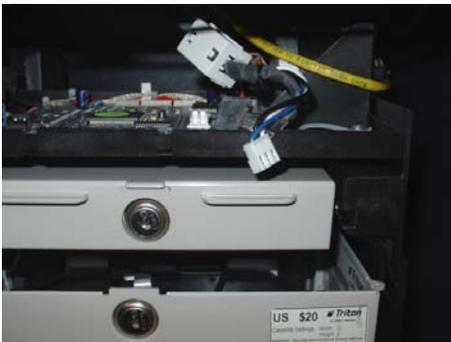
Figure 4. Power and Comm cable disconnected.
