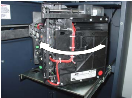
Figure 3. Rotate mechanism to service position (clockwise).
