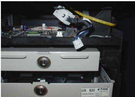
Figure 5. Power and Comm cable disconnected.
