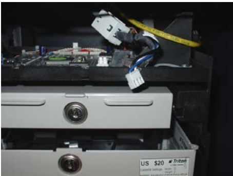
Figure 4. Power and Comm cable disconnected.
