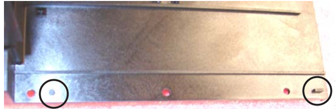
Figure 6. Align base plate with notches.
