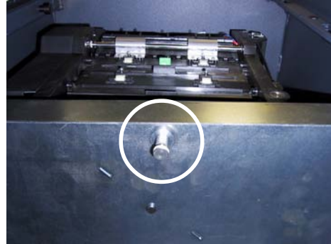
Figure 2. Pull release pin for swivel platform.
