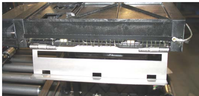
Figure 1. Place brush above currency exit slot.
